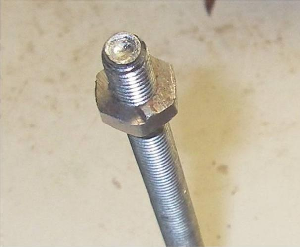
The threaded bar is fixed to the lathe with the chuck. Place the wooden insert onto the threaded bar and hit the opposite end with a hammer so that the nut penetrates into the insert and this will prevent it from moving when the chuck rotates.
