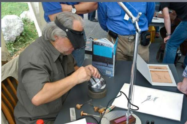
Jaroslav demonstrated us how to engrave a ferrule by using a special turning vise and a hand graver.
