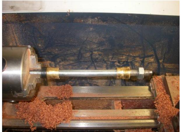
A threaded bar with spacers onto which the insert can be placed and a nut to tighten everything and that can be placed into the chuck jaws.
