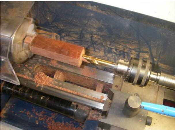
The bit does not rotate and chips tend to accumulate in the drills grooves and this causes the wood to overheat. Stop often to get rid of the chips.
