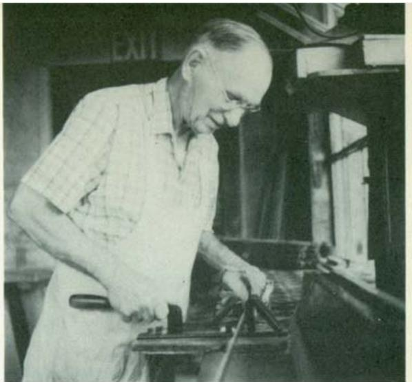
Cito le sue parole come appaiono nel suo catalogo del 1951 “Before filling down the nodes or raised joints on the cane, we employ an extra straightening process so that only a small projection is left to be filled off and the vital hard surface fibers are not cut away in the wide area adjacent to the node.”
