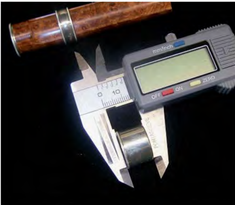
External measurement (put value in F/RS Ext);
