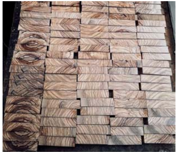
Seasoned billets of Tuscan olive wood ready to be turned and shaped for reel seat fillers. Olive wood, cut across the grain, is all we use. It's incredibly hard, very highly figured and a feature of our fly rods.
