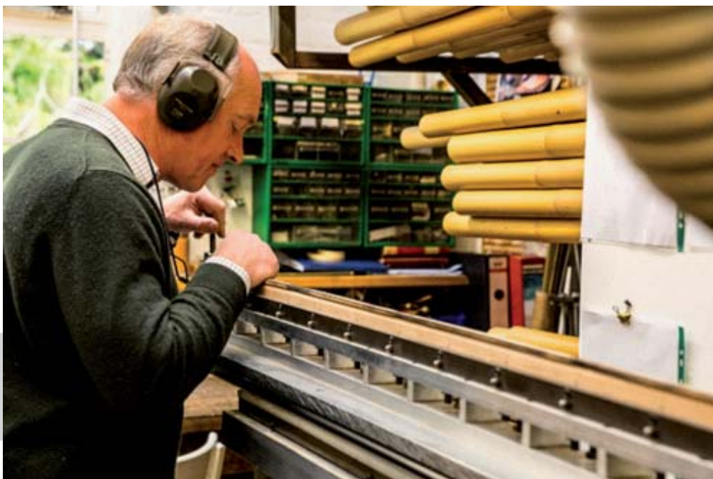
Clamping a bamboo strip to the carriage of the milling machine
