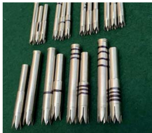
Nickel silver ferrules with splint ends and waterproof caps, made by Colin to H L Leonard's design of 1878
