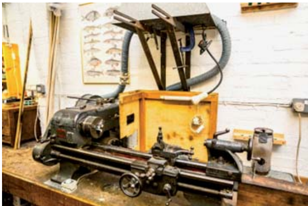
The pre-1939 Chicago built Logan lathe that we use for turning reel seat inserts, ferrule stoppers & cork handles.
