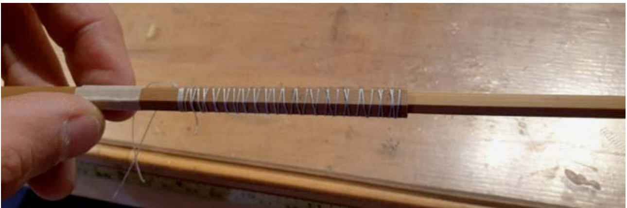
Wrapping/whipping a hex TBF ferrule during gluing of the tip
