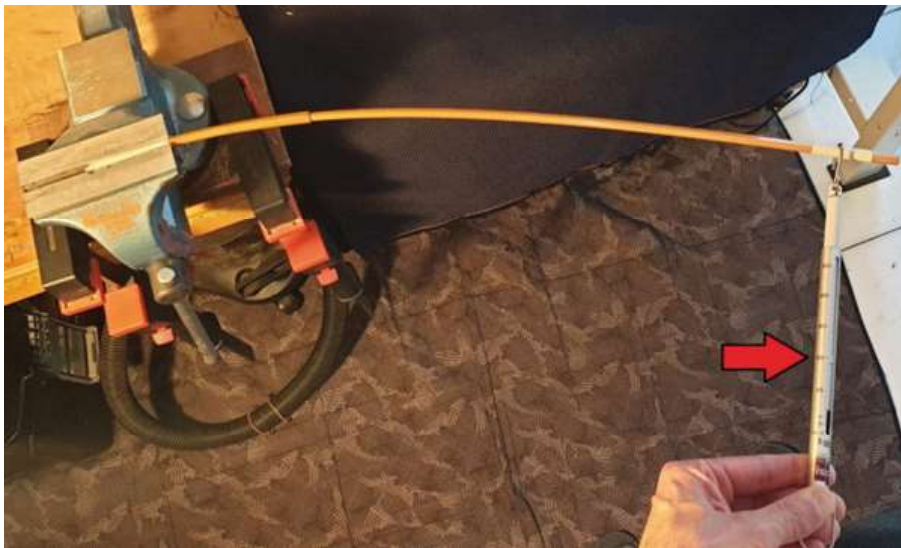
Load test up to 1kg (2.2lb) on TBF sample
