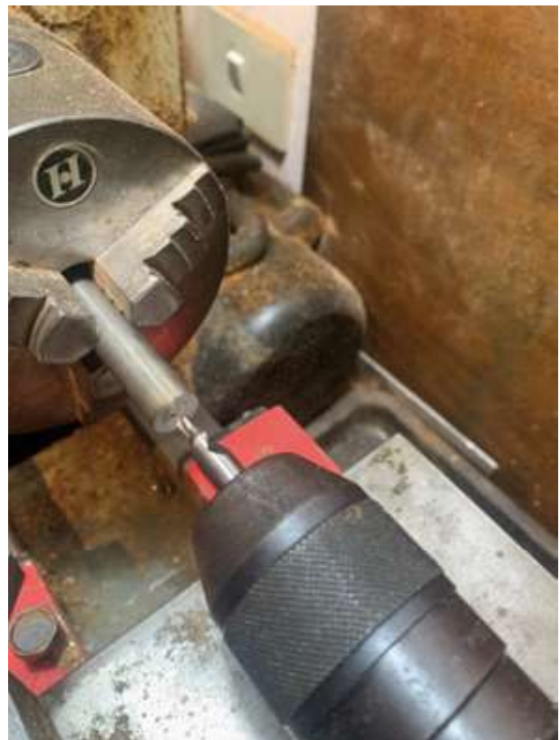
Round bar stock just before the centre hole
